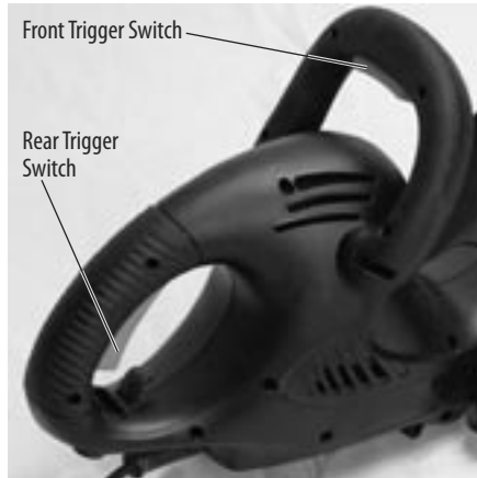
Figure 3-5: Front and rear trigger switches
